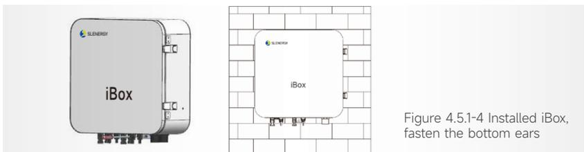
Figure 4.5.1-4 Installed iBox, fasten the bottom ears
